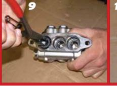
Hi-Pressure Seal is easily removed from the manifold without any tools. If extremely worn a reverse pliers may be used.
