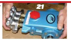
V-Packing models or larger manifolds it may be necessary to gently tap with a soft mallet until the manifold is flush with the Crankcase. Replace (2) Lockwashers, (2) Socket Head Screws and torque per chart.
