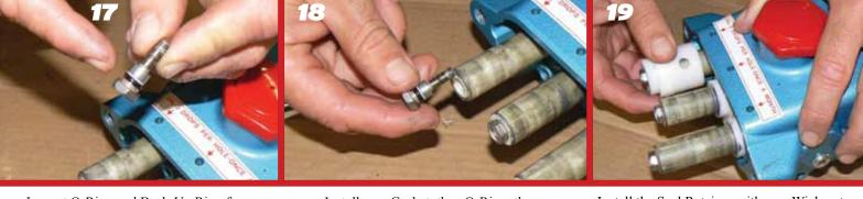
Inspect O-Ring and Back-Up Ring for wear & replace if needed. Examine Ceramic Plunger for scoring, scale build-up, chips or cracks and replace if needed.
