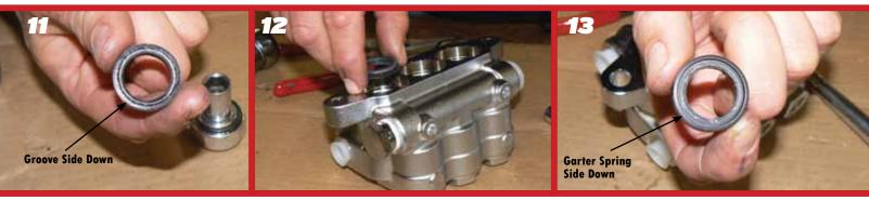
Carefully square Hi-Pressure Seal into position by hand with the **grooved side down**.
