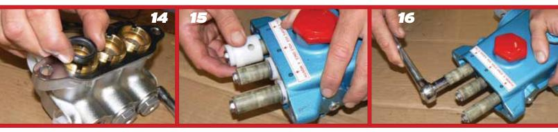
Install Lo-Pressure Seal into each seal case with **Garter Spring down**.
