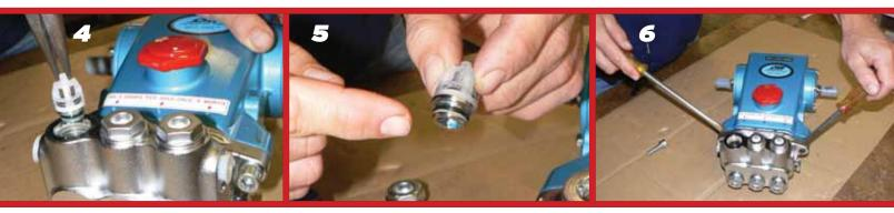
Grasp Spring Retainer by tab at the top with pliers and remove from valve chamber.
