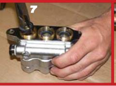
Place Manifold Head on work surface with **crankcase side up.** *Remove Lo-pressure Seal On 5PFR & 7PFR plunger pumps prior to May 1989, remove Snap Ring & Lo-Pressure Seal from each Seal Case. Discard Snap Rings. On 5PFR & 7PFR plunger pumps after May 1989, remove Lo-Pressure Seal from each Seal Case.*
